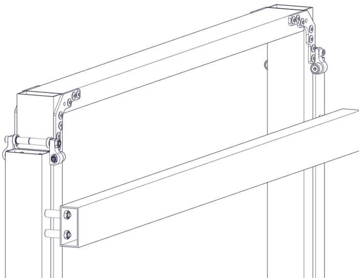
Do NOT make this assembly too tight! The inner carriages should freely and smoothly move inside the outer frame. If this proves too challenging to assemble in this fashion, you can remove the cam followers on one side to remove the inner carriage and then replace it when completed.
